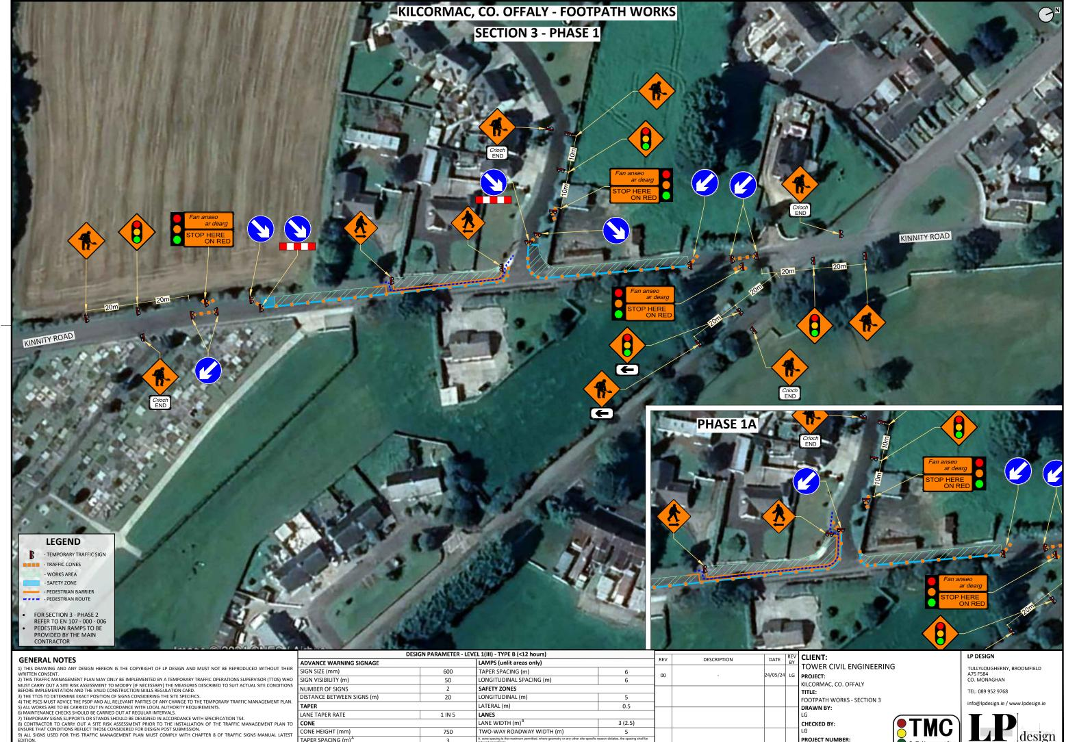
10) SAFETY BARRIERS USED FOR THIS TMP MUST COMPLY WITH TII DN-REQ-03034-1 IS EN 1317-1 E) TEMPORARY SAFETY BARRIER.
