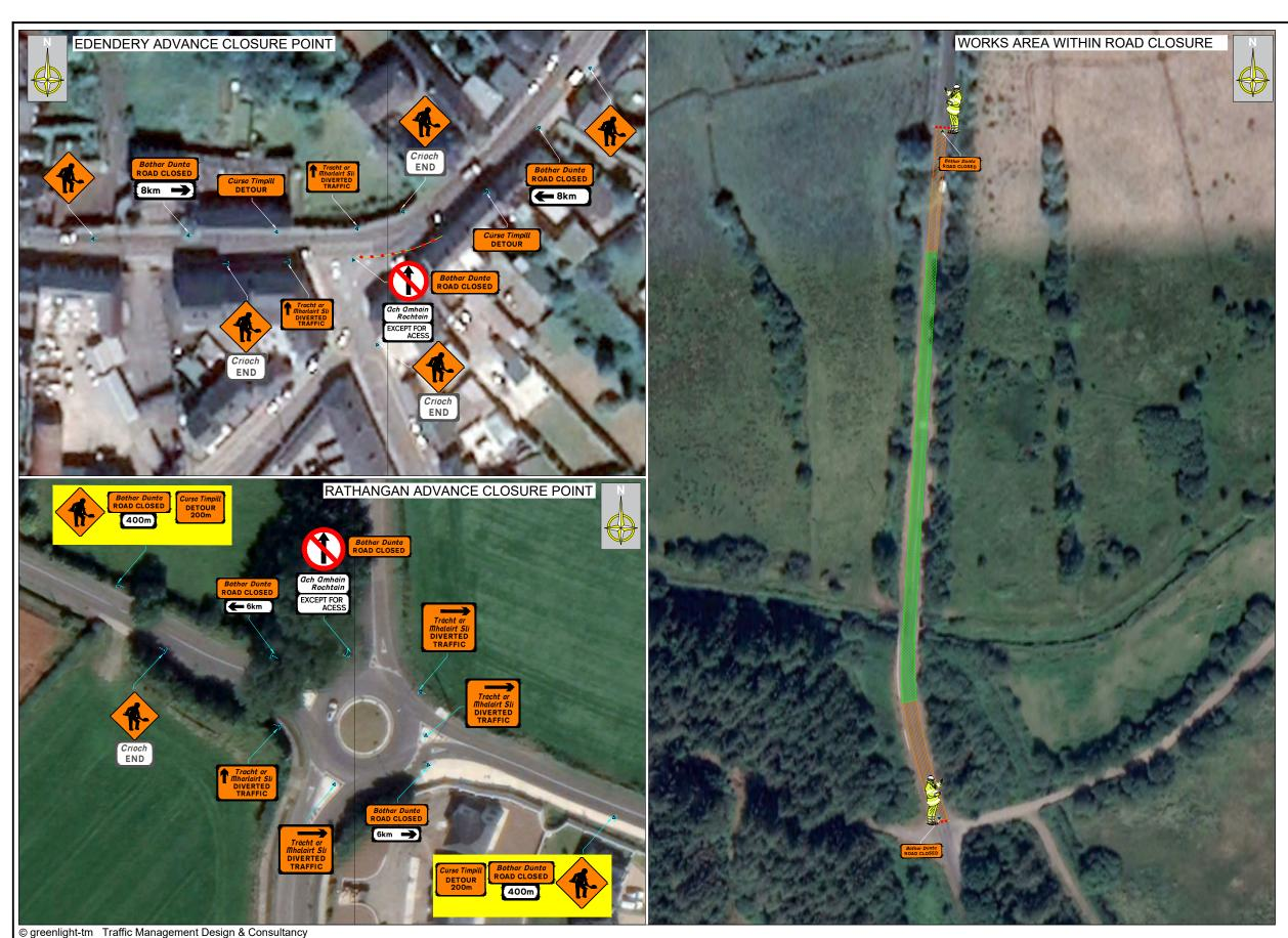
TYPE A >12 hours Sign Size (mm) 600 Sign Visibility (m) 90 No. of Signs Cumulative Distance (m) Distance between Advance 120 Warning Signs (m) Taper Lane Taper Rate 1 in 40 1 in 40 Hard Shoulder Taper Rate 750 Taper Spacing (m) Longitudinal Spacing (m) Taper Spacing (m) Longitudinal Spacing (r Longitudinal (m) 1.2 Lanes (minimum Lane Width (m)
