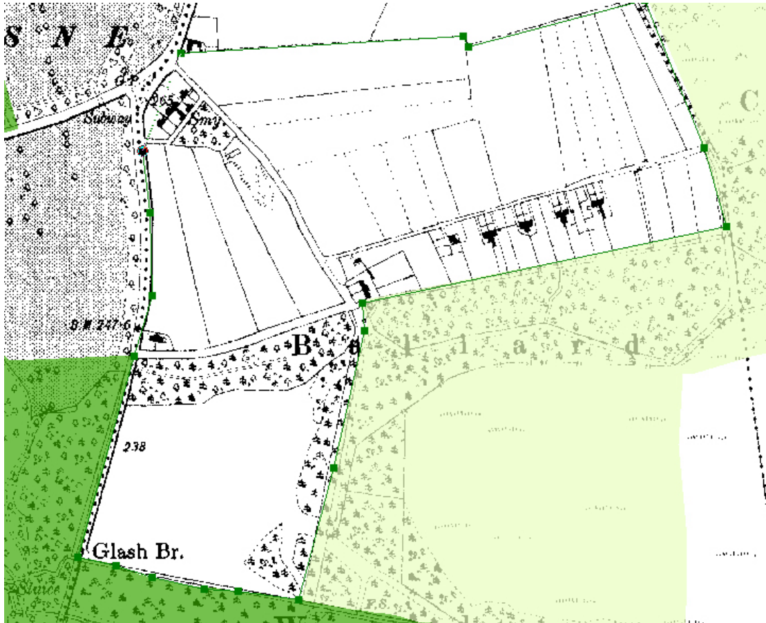
Fig 3.2: Creation of a HLC polygon using 3 rd edition map sources and the inclusion of 1:50,000 OSI data within the creation of the HLC map.
