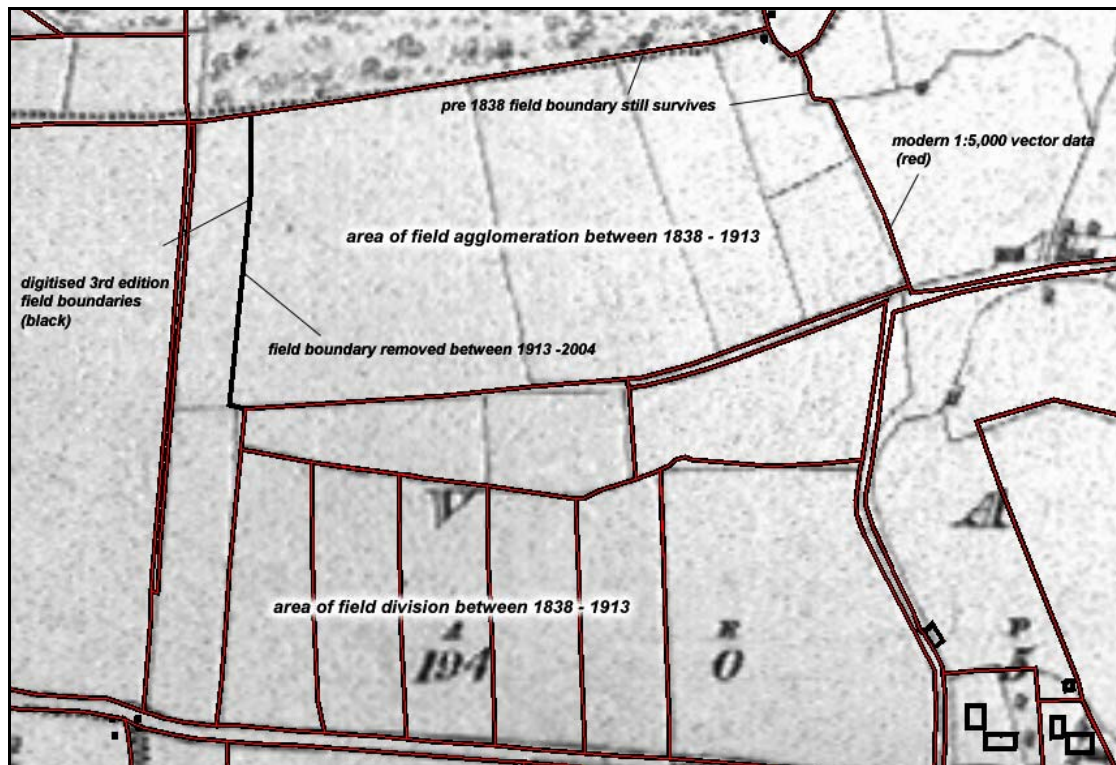
Figure 5.7: Illustration of a geo-referenced 1 st edition map and its relationship to field boundaries created in stages 2 and 3.
