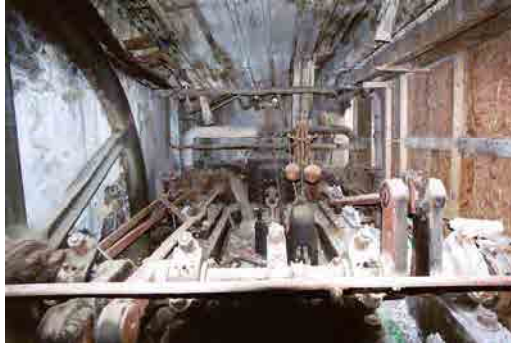
OFIAR-017-036_13 FWH 16/07/2003 Building 2: steam engine detail showing valve box and cylinders.
