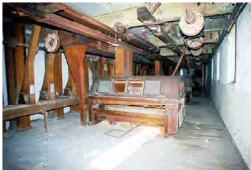
OFIAR-008-038_27 FWH 15/10/2003 Second floor of east section of mill, looking north. Note purifiers.
