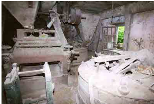
OFIAR-016-002_08 FWH 09/06/2003 Millstones and roller mill on first floor of mill.
