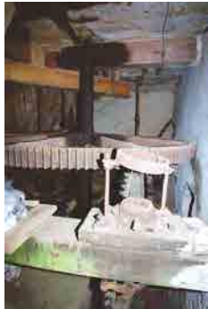
OFIAR-014-004_16 FWH 24/06/2003 Oat mill power transmission gearing.
