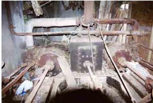
OFIAR-017-036_13 FWH 16/07/2003 Building 2: steam engine detail showing valve box and cylinders.
