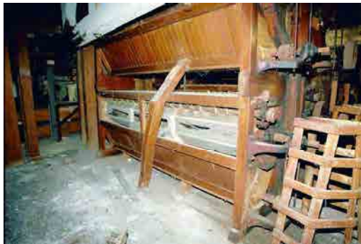
OFIAR-008-038_30 FWH 15/10/2003 Centrifugal sifter on third floor of east section of mill.
