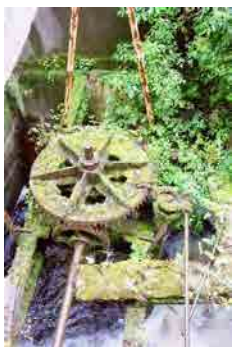
OFIAR-016-002_03 FWH 09/06/2003 Crown wheel on top of turbine rotor shaft.
