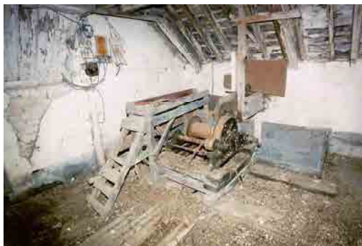
OFIAR-031-012_08 FWH 31/07/2003 Electric sack hoist at north-west end of top floor of malting.
