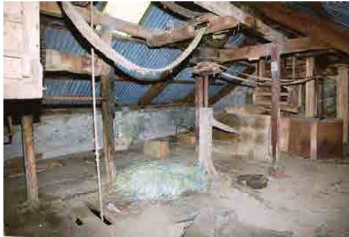
OFIAR-009-006_08 FWH 11/06/2003 Mill: top floor with sack hoist at left and oatmeal sieves/fans at right.
