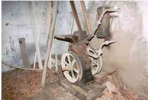
OFIAR-009-005_16 FWH 11/06/2003 TVO engine in cascade dryer room.
