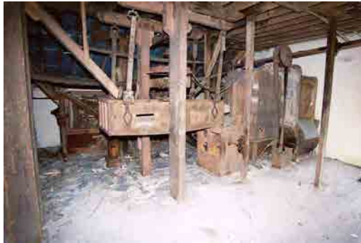
OFIAR-014-004_20 FWH 24/06/2003 Oat mill fourth floor showing reciprocating sieve and aspirator.
