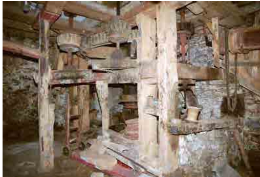
OFIAR-009-006_04 FWH 11/06/2003 Mill: power transmission shafts and gears on ground floor.
