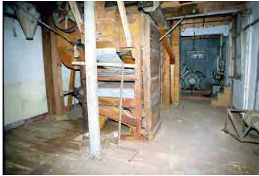
OFIAR-008-038_22 FWH 15/10/2003 Scourer on second floor of west section of mill.
