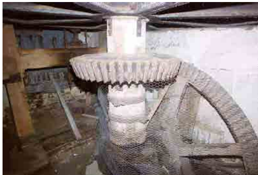
OFIAR-043-002_10 FWH 18/07/2003 Mill: Pitwheel, wallower and upright shaft on ground floor of east bay.
