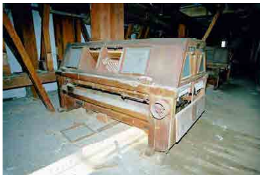
OFIAR-008-038_28 FWH 15/10/2003 Semolina purifier on second floor of east section of mill.
