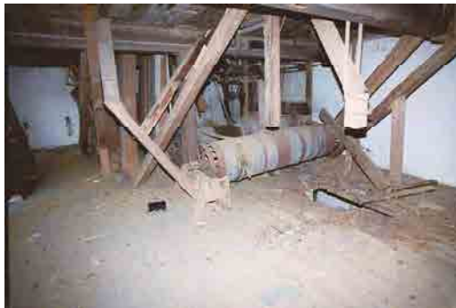
OFIAR-014-004_18 FWH 24/06/2003 Oat mill second floor. Note cylindrical separators.
