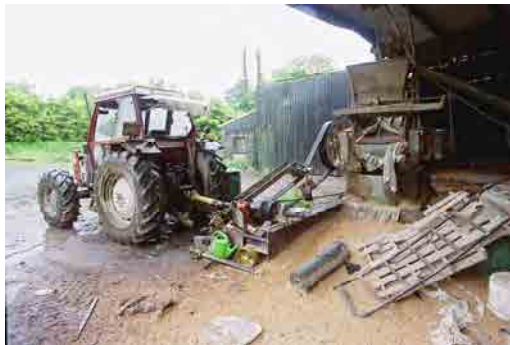
OFIAR-016-002_12 FWH 09/06/2003 Modern tractor-driven roller mill in adjoining shed.
