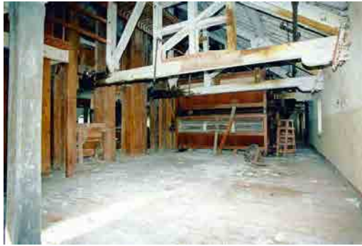
OFIAR-008-038_30 FWH 15/10/2003 Centrifugal sifter on third floor of east section of mill.
