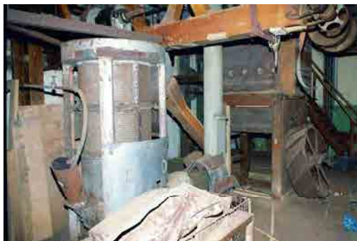
OFIAR-008-038_20 FWH 15/10/2003 Whizzer (left) and conditioner-dryer on ground floor of west section of mill.
