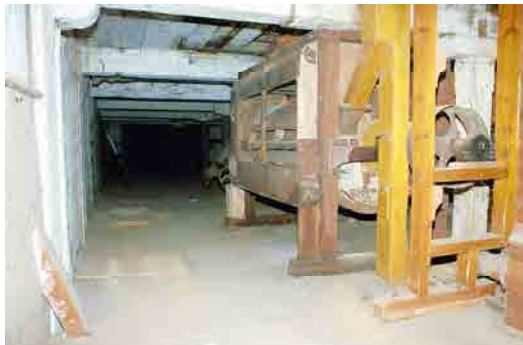
OFIAR-008-038_22 FWH 15/10/2003 Scourer on second floor of west section of mill.
