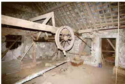
OFIAR-009-005_13 FWH 11/06/2003 Lineshaft drive and sack hoist on top floor of store.
