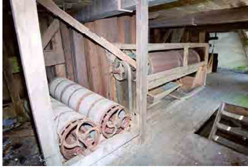
OFIAR-014-004_20 FWH 24/06/2003 Oat mill fourth floor showing reciprocating sieve and aspirator.
