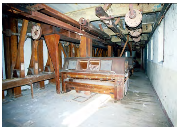
Fig 2.19 Semolina purifier in Erry Mill (008-038).
