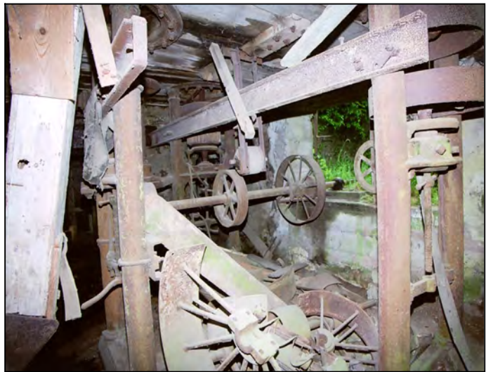
Fig 7.12 Derelict power transmission shafts and pulleys at Ballyduff Mill.
