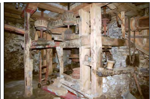
Fig 2.13 Left: Two-step transmission system to multiple sets of stones.
