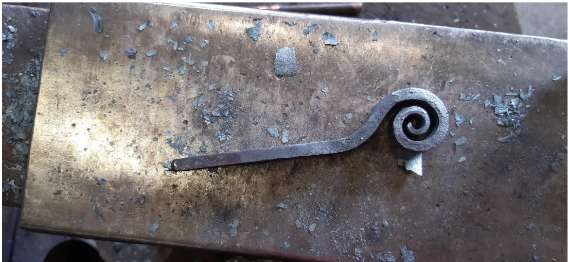
Stages in forging the scrolls
