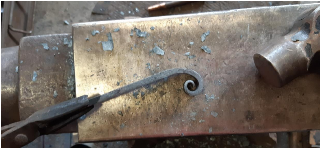
Stages in forging the scrolls
