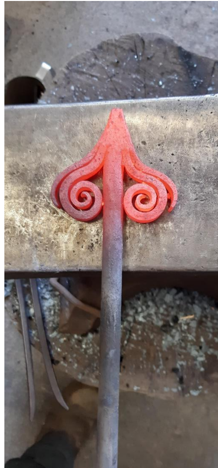
Ribbons and scrolls being arranged and fire welded to make a replacement finial
