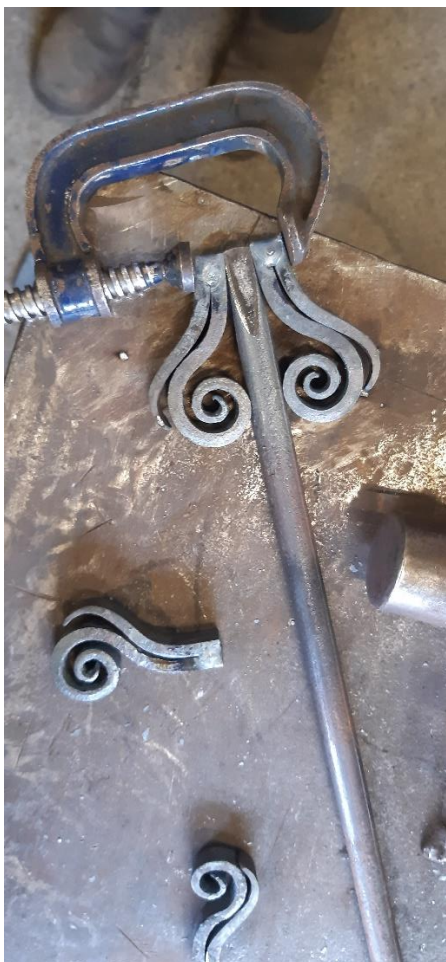
Ribbons and scrolls being arranged and fire welded to make a replacement finial
