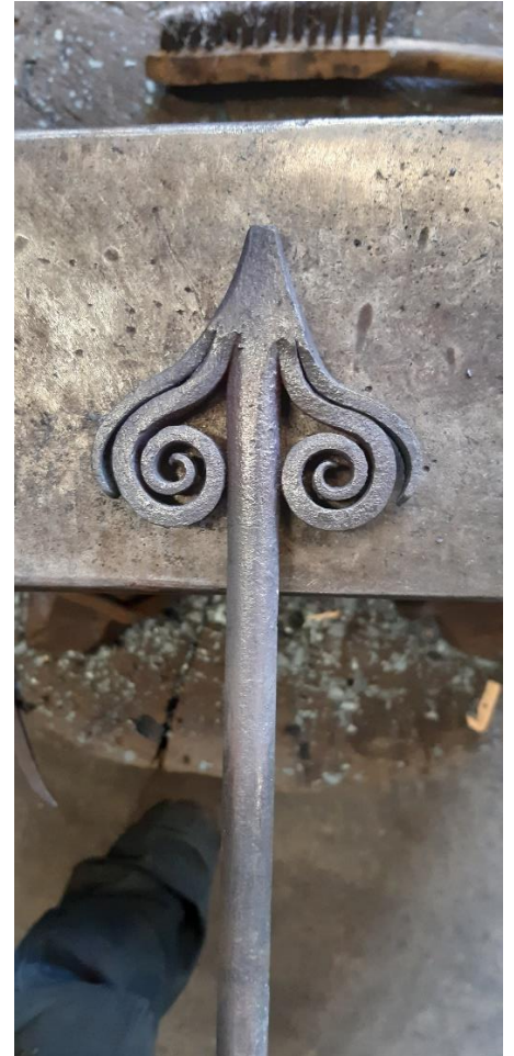
Ribbons and scrolls being arranged and fire welded to make a replacement finial
