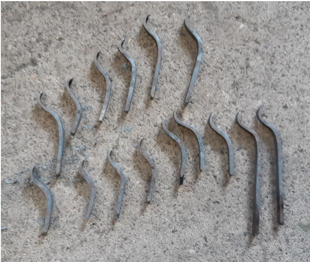
New ribbons forged from wrought iron
