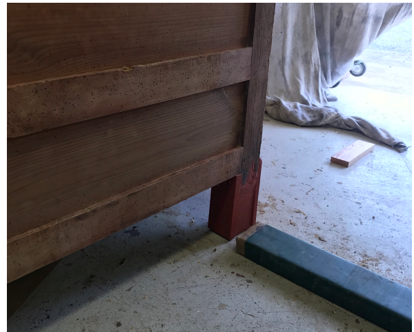
Beech extension fixed inside supports
