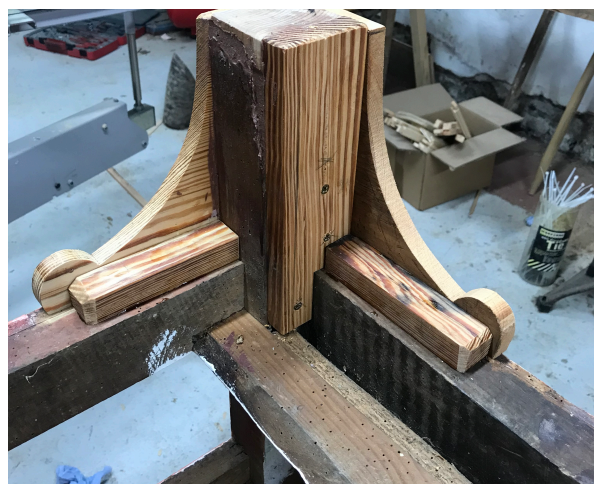
Corner blocks rub jointed to rear of feet.
