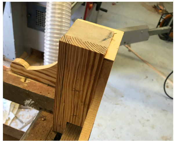
Beech extension fixed inside supports
