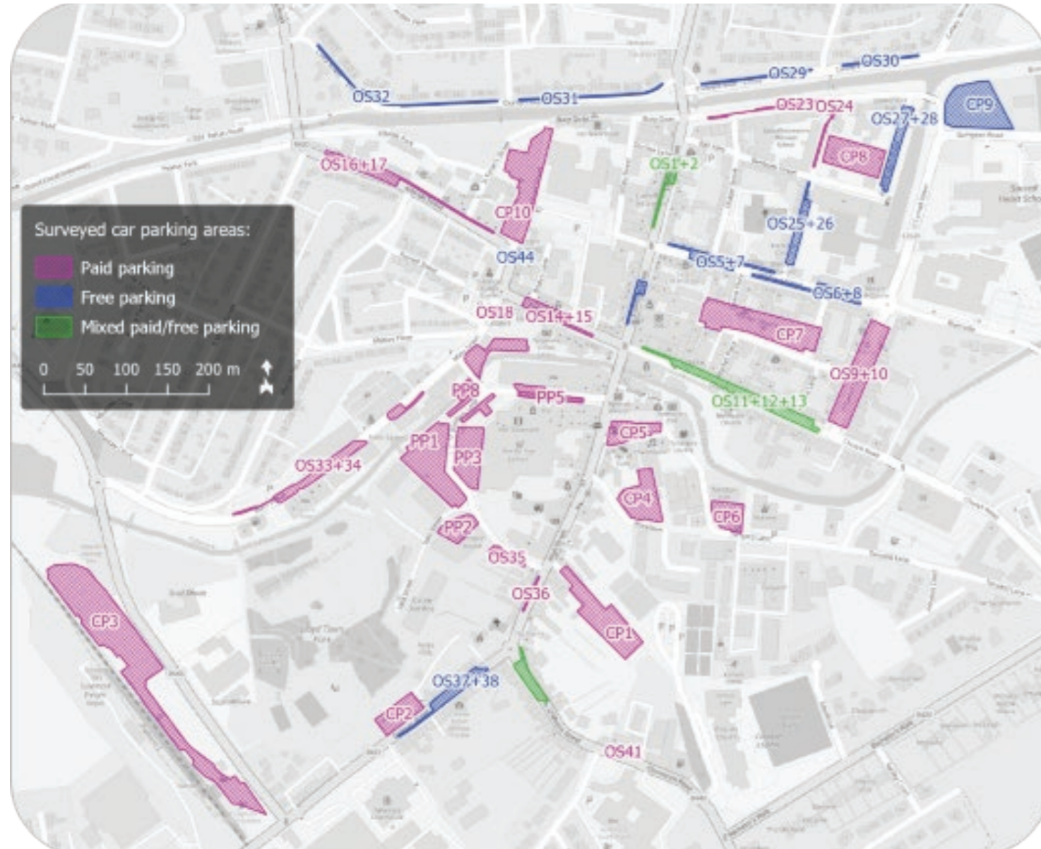
Figure 15 – Surveyed car parking areas (with ID codes) (background map imagery: OSM Contributors)
