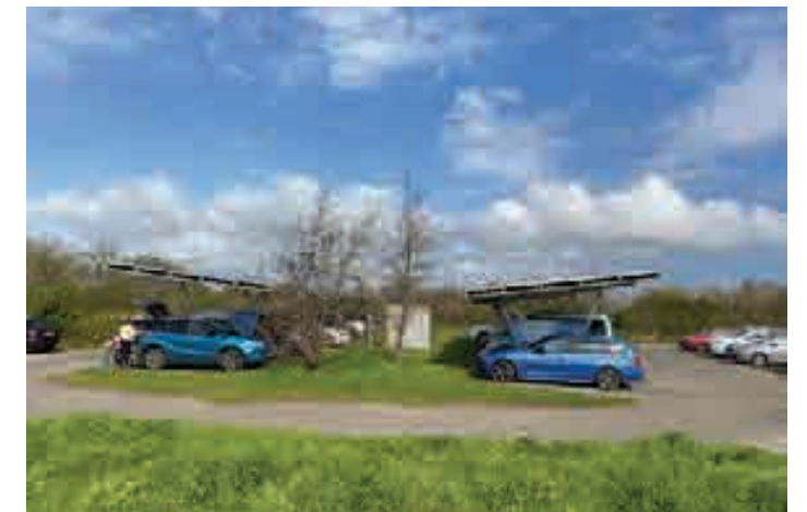
Above: the car park and pathways at Lough Boora use primarily natural materials and are permeable. Integrating solar PV shelters in some bays will help power the site..
