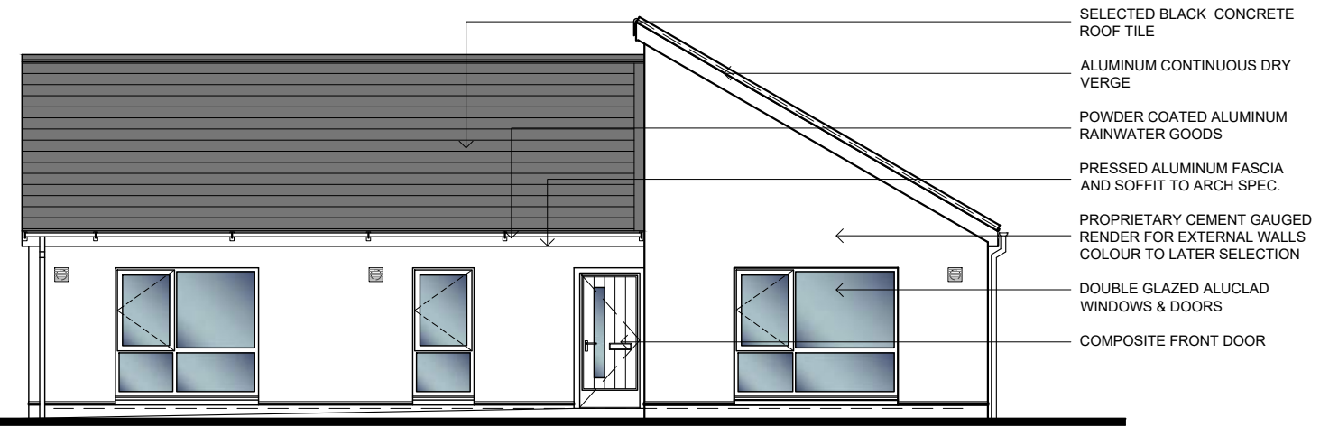
4 Bed Bungalow: Front Elevation 1:100 @ A3
