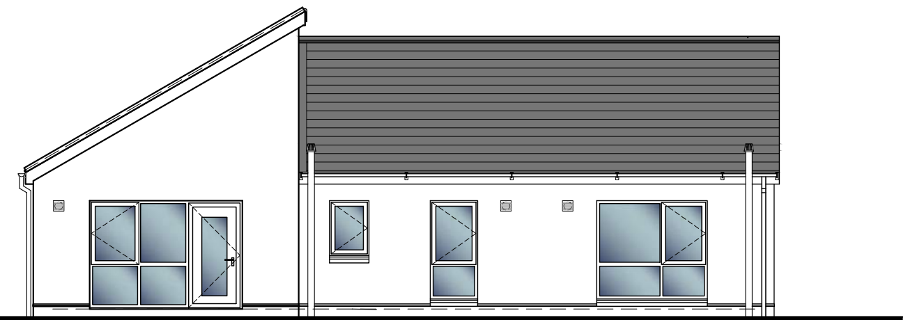
4 Bed Bungalow: Rear Elevation 1:100 @ A3
