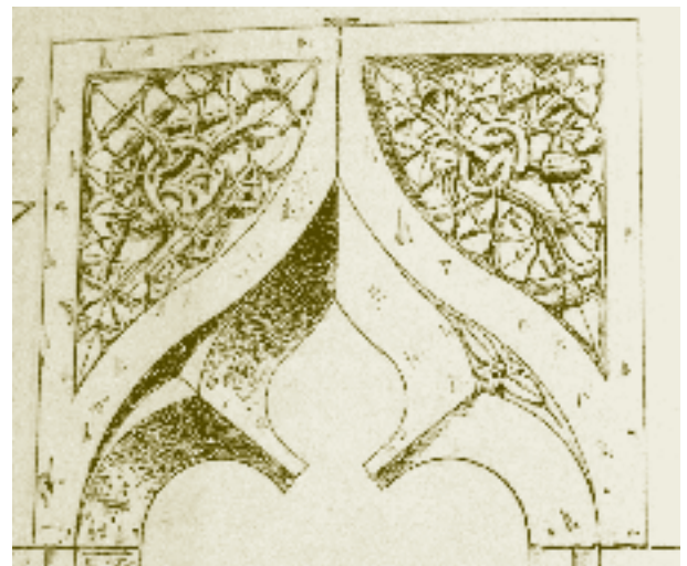
FIGURE 25. Drawing by William Martin of head of single light ogee-headed window in north wall of nave with spandrels decorated with vine-leaf carvings (1911).
