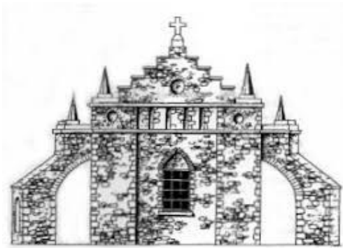
Bellevue Gothic Cottage, Lawrencetown, Co. Galway – built possibly circa 1782 with other Gothic aspects of estate. One of few examples of flying buttresses used in garden buildings in Ireland.
