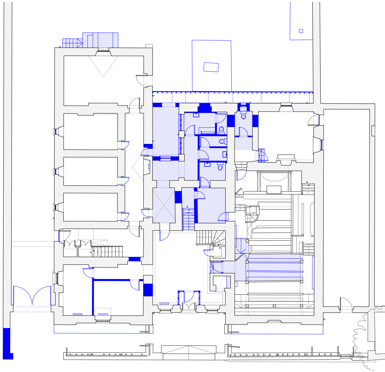
Figure 49 - Existing/Demolition Ground Floor Plan
